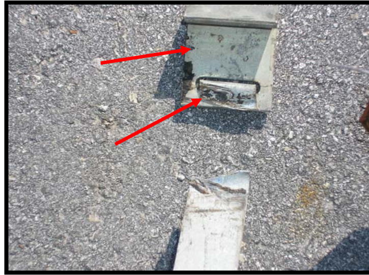
I-beam hooks were used and had no radius clips.
